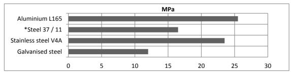
\*Steel 37 / 11: tested with adhesive joint thickness of 1 mm, the performance may be lower for thinner adhesive joints.
